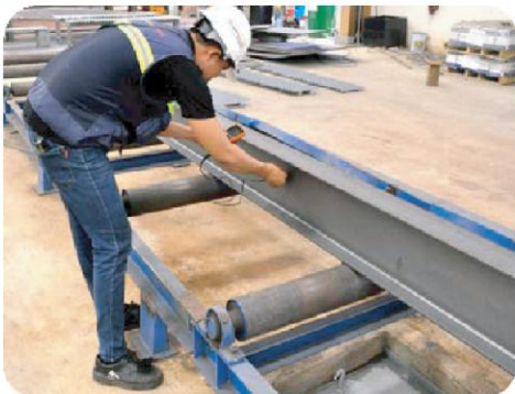
SHOT BLASTING CHECKING
