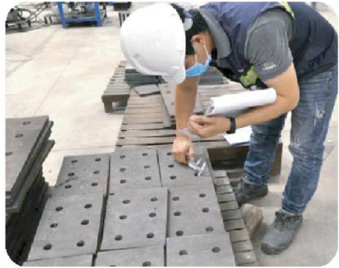
DRILLING & CUTTING CHECKING
