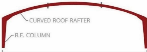
CURVED ROOF RAFTER R.F. COLUMN MAX . PRACTICAL WIDTH = 90 Mtr. ARCHED CLEAR-SPAN (AS)
