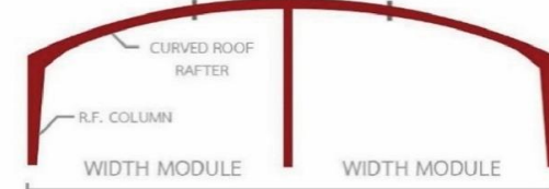
CURVED ROOF RAFTER R.F. COLUMN WIDTH MODULE BUILDING WIDTH MAX . PRACTICAL WIDTH MODULE = 70 Mtr. MORE MULTI - SPANS ARE POSSIBLE (AMS-2, AMS-3,...) ARCHED MULTI - SPAN (AMS-1)
