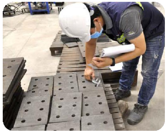
DRILLING & CUTTING CHECKING
