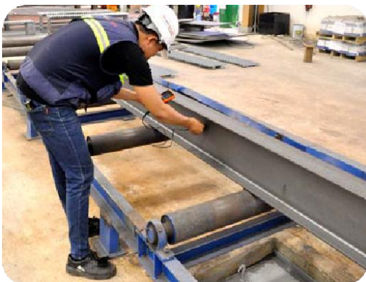
SHOT BLASTING CHECKING
